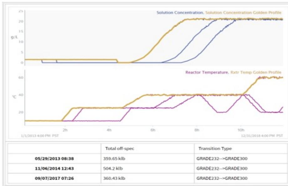
Seeq screenshot shows how three of the shortest product transitions were combined to create a golden profile summarizing the set point adjustment rates recommended for operations to minimize the overall transition time period.
