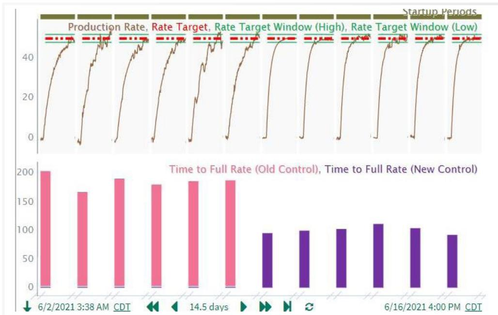
Shown in the picture: Visualization of decreased time to full (target) rate for automatic control improvements in Startup Periods. We can see in Seeq Chain View that time has decreased from 150-200 minutes to approximately 100 minutes.
